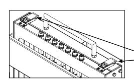
6. Hold the Flame Unit and body in one hand, and lock the Snap Lock in the other.
