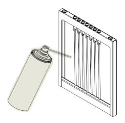
1. Spray the attached oil on the Blade.
