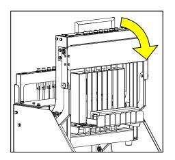
3. Hold the Handle with both hands tightly.Pull the Handle forward quickly.
