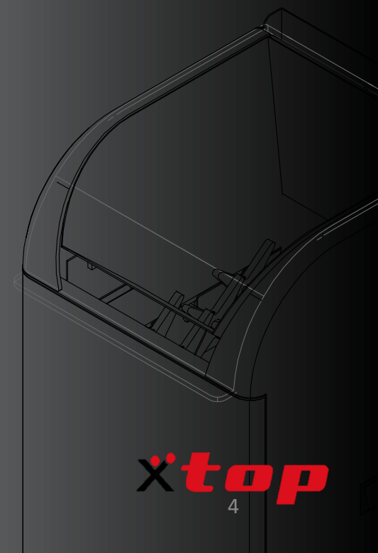
SAFETY It is safe because it stops when the front cover is opened.
