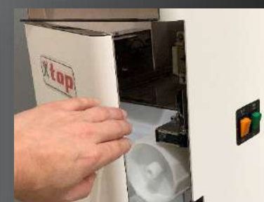
SAFETY It is safe because it stops when the front cover is opened.
